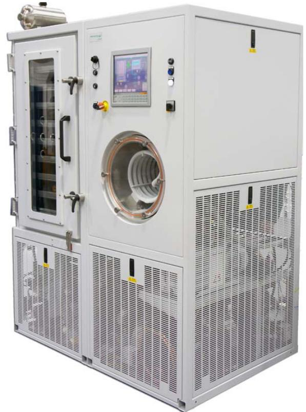
LSG60 LyoDry Grande has nine temperature controlled shelves, between ±60°C with an accuracy of better than ± 0.5°C.
