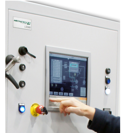
User friendly interface with 200 retrievable process profiles
